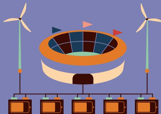
The purpose of this energy storage system is to supply the stadium with sufficient electricity from renewable sources, such as solar or wind energy. If the weather changes and the wind and sun stop playing along or if demand spikes during a game, the e-battery steps in and balances the power supply.
