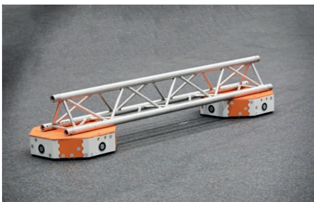
Figure 20: Collaborative transportation of a crossbeam (source: Michael Neuhaus/Fraunhofer IML)
