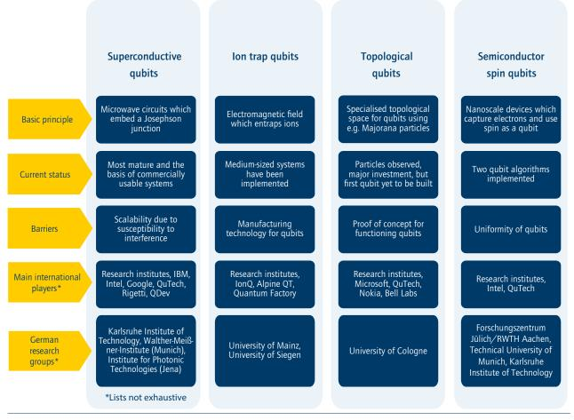
Figure 20: Overview of different approaches to the implementation of a quantum computer (source: own presentation based on Birch 2018)
