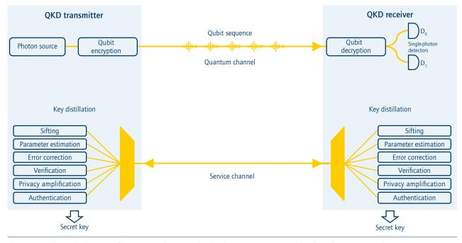
Figure 11: Schematic diagram of QKD-secured communication (source: own presentation based on ETSI 2015)
