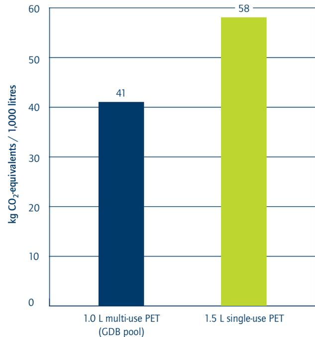
Figure 21: Comparison of greenhouse gas emissions of multi-use PET and single-use PET (Source: own presentation, based on: ifeu 2020)
