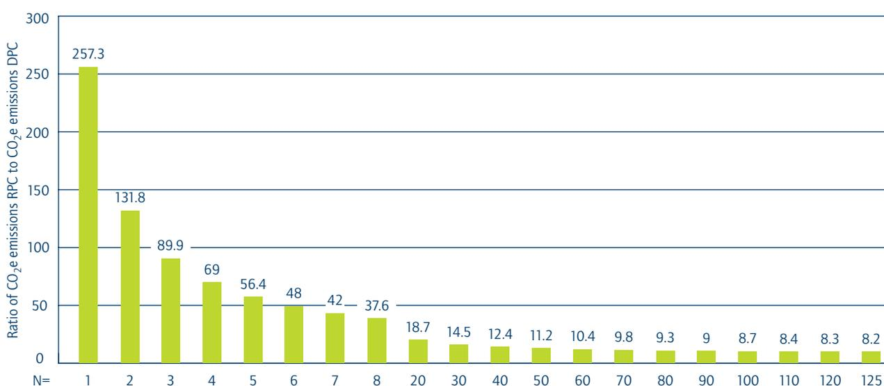
Figure 20: Emission of CO<sub>2</sub> equivalents from RPCs in comparison with DPCs (Source: Tua et al. 2019)
