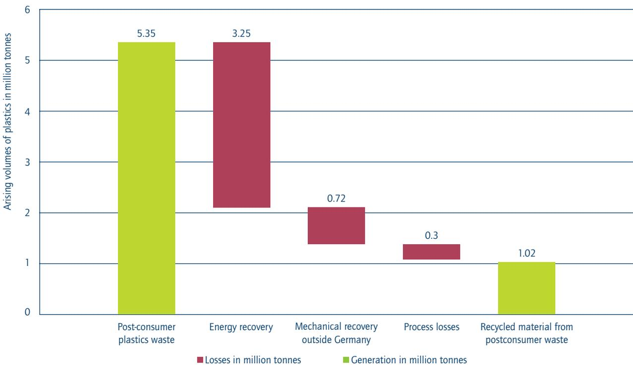
\* Due to the small volumes involved, the graph does not show losses due to landfilling (~0.03 million tonnes), feedstock recycling (~0.01 million tonnes) and export surplus (~0.01 million tonnes)
