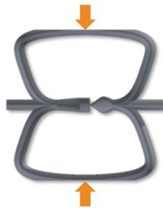
Figure 36: Individual elements can be enabled through their internal molecular or mesoscopic structure to respond to external stresses (arrows). The figure shows an individual element which has been designed to become soft as foam under a light load and rigid as wood under a heavy load (source: Matthew Berwind, Fraunhofer Institute for Mechanics of Materials IWM/University of Freiburg).
