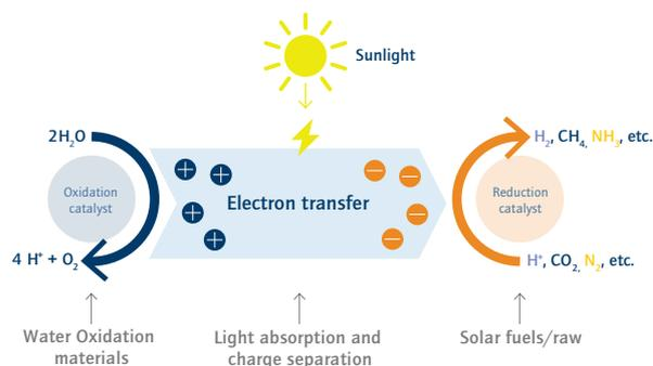
Figure 18: Overview of sub-processes of Artificial Photosynthesis (source: acatech et al. 2018)
