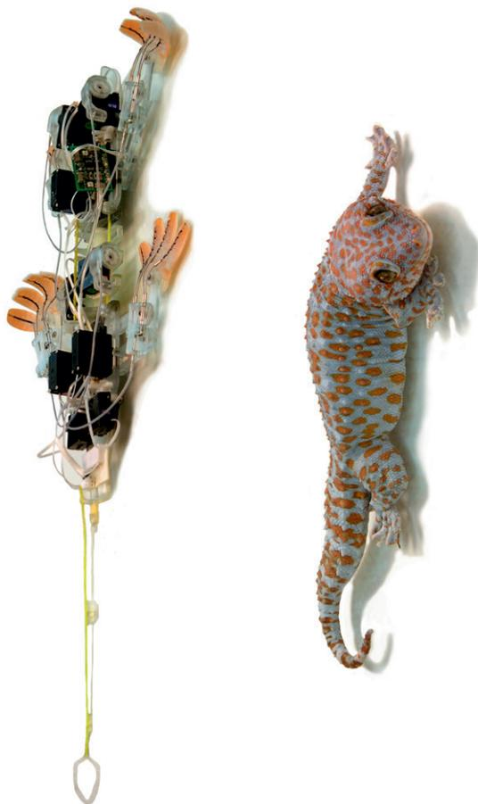
Figure 54: A gecko-inspired robot named "Stickybot" climbing next to its inspiration, the tokay gecko that uses a fibrillar adhesive (source: Robert J. Full, UC Berkeley)
