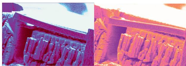
Figure 7: Micromanipulator experiment with a  $3 \times 3 \mu\text{m}^2$  beam of mesocrystalline cement. On the left, before the experiment; on the right, marked flexure of the beam under pressure without breakage. After deformation, the beam returns to its original position (left), revealing advantageous elastic deformation; all the energy is reversibly returned (source: Helmut Cölfen, University of Konstanz).
