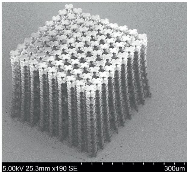
Figure 37: Mechanically programmable metamaterials consist of many individual elements which interact in concerted manner to perform system functions (source: Fraunhofer Institute for Mechanics of Materials IWM).
