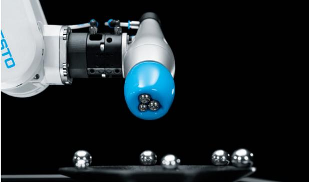
Figure 16: Inspired by the chameleon's tongue, the FlexShape-Gripper is capable of grasping a huge range of objects by moulding itself around them (source and copyright: Festo AG & Co. KG, all rights reserved).
