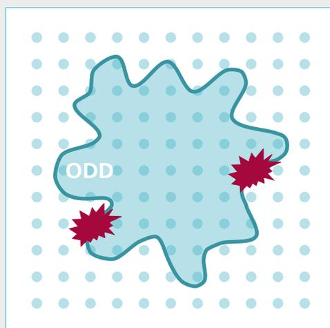
Note: The **Operational Design Domain** (ODD) describes the boundary within the set of possible operating conditions. Possible corner cases (red symbols) often occur in the marginal areas of the parameters.
