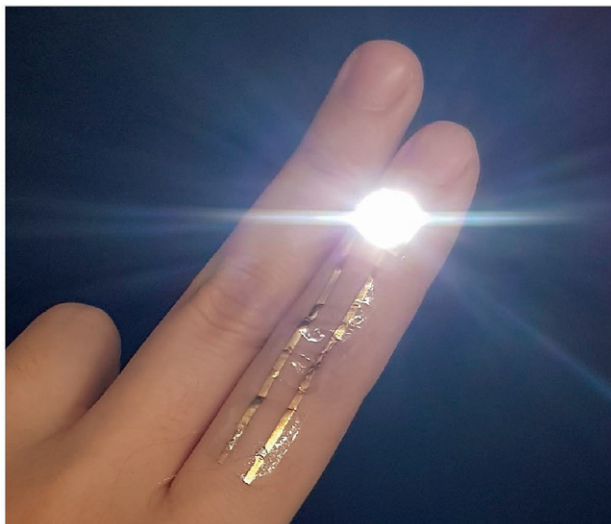
Figure 55: On-skin, silk-based electrodes with high skin conformability and high conductivity developed by Prof. Chen and his group (source: School of Materials Science and Engineering, Nanyang Technological University)
