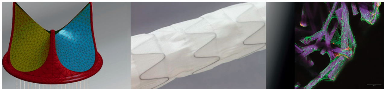
Figure 35: A perfused geometric structural model of a woven heart valve (left), an integrally fabricated stent graft with stent rings woven into the prosthetic structure (graft) (centre) and a fluorescence micrograph of a bio-inspired short-fibre scaffold (source: Institute of Textile Machinery and High-Performance Material Technology, Dresden)
