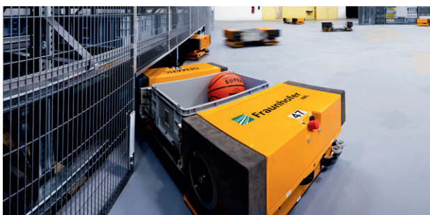
Figure 39: Cellular transport system with decentralized multi-agent control, in which software agents represent the individual vehicles and negotiate transport orders and routes, autonomously (source: Fraunhofer Institute for Material Flow and Logistics IML)
