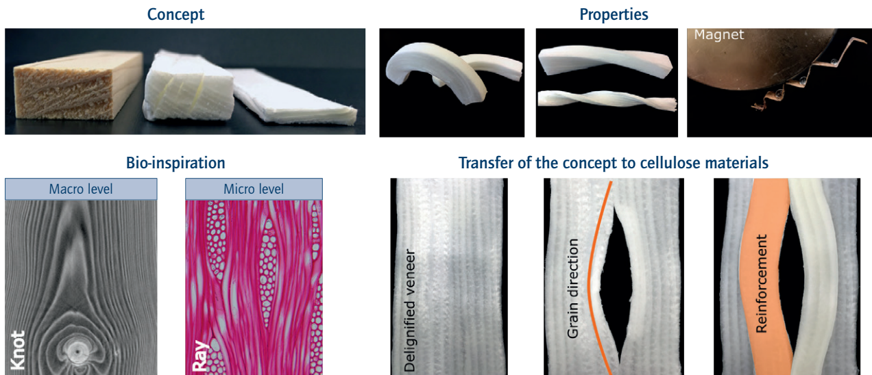
Figure 11: Cellulose composites based on a synthesis of bio-inspiration with use of the renewable resource which is wood in modified form (source: in part from Frey et al. 2018 and Frey et al. 2019)
