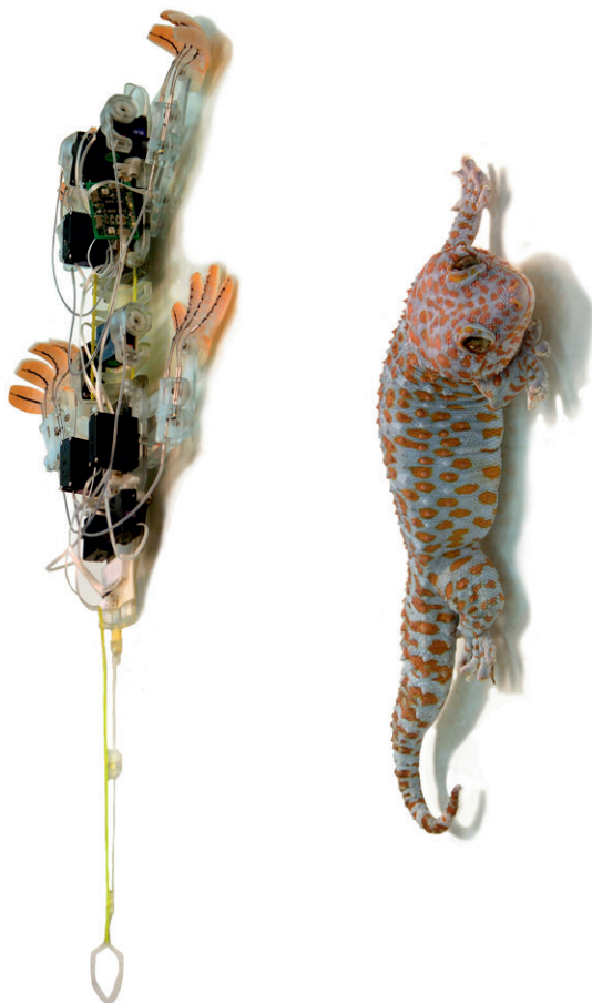
Figure 54: A gecko-inspired robot named "Stickybot" climbing next to its inspiration, the tokay gecko that uses a fibrillar adhesive (source: Robert J. Full, UC Berkeley)
